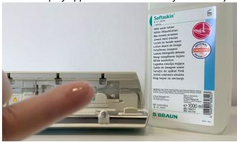
3. Bring the Softaskin® onto the peristalsis of the pump and distribute it evenly in the marked area. Softaskin® must not be brought onto air sensor above the yellow warning light.
