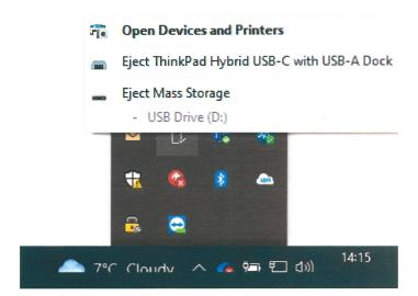
Eject the USB device (this is important) and remove it from the PC. It is now ready to be used to upgrade Team3 units to version 19.4
