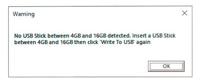
If the USB memory stick contains log files created during an upgrade operation, the following message is displayed when trying to write the upgrade files:
